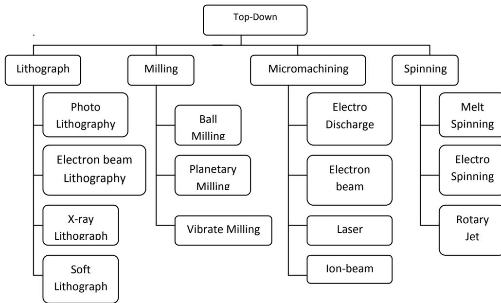
Figure (1) Classification of e common top-down methods for nanostructured material synthesis (Liu. et al., 2008,pp331-336).
