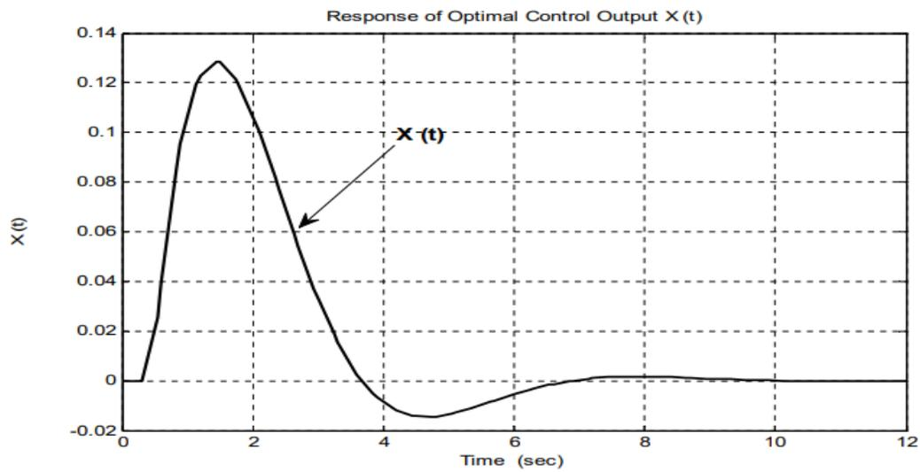
Figure 3-2: Closed loop System response (input signal is impulse).
