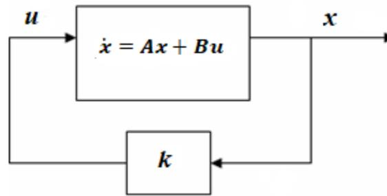
**Figure 2-1:** Optimal Regulator System.
