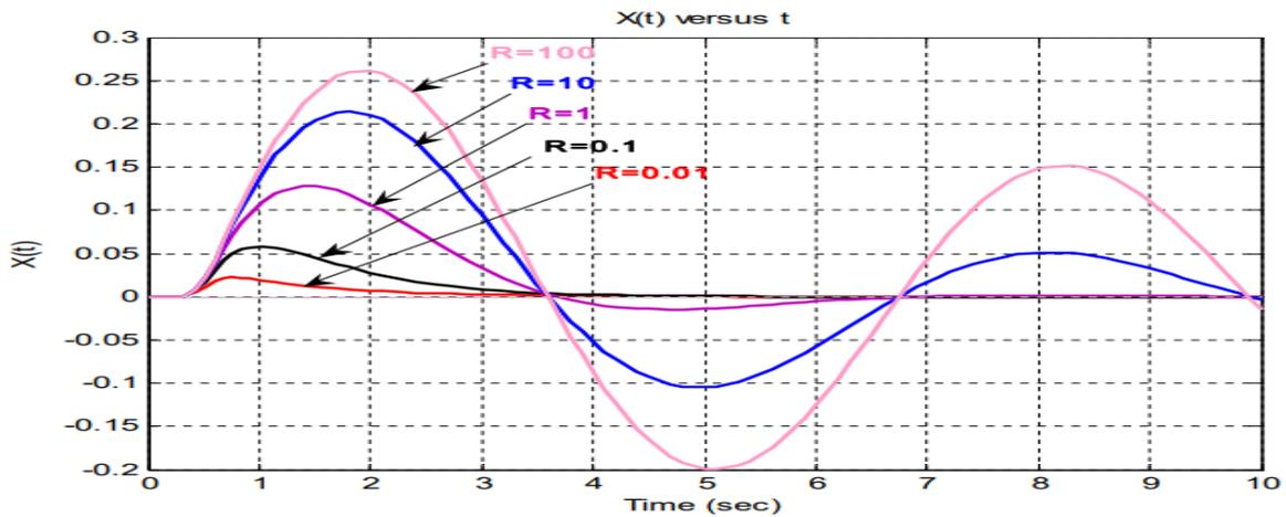
Figure 3-4: Closed loop System response with different values of R.
