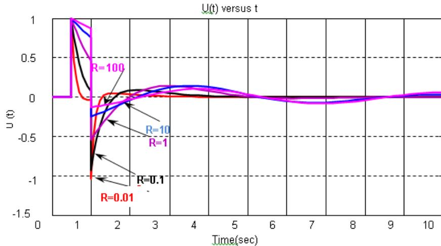
Figure 3-3: Closed loop System response with different values of R.
