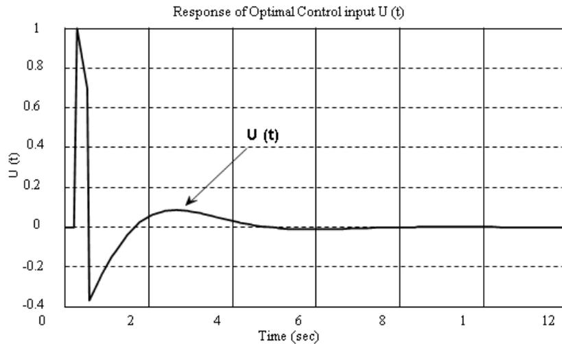
Figure 3-1: Closed loop System response (input signal is impulse).
