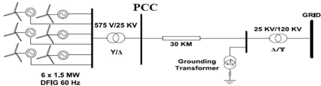
Figure 2 shows the studied system, which consists of six 1.5 MW DFIGs connected to the ac grid at the PCC. The grid that is represented by an ideal three-phase voltage source of constant frequency is connected to the wind turbines via 30km transmission line and step-up transformer. The proposed SMES unit and STATCOM are connected to the PCC via a coupling transformer.
