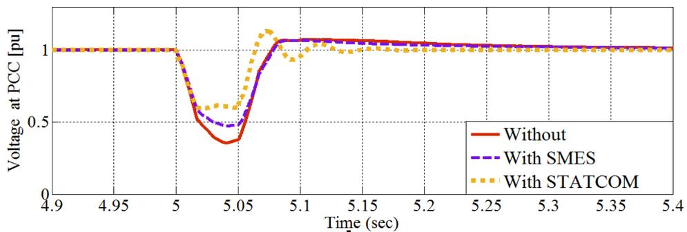
Figure 8: PCC voltage compliance with Garman grid code
