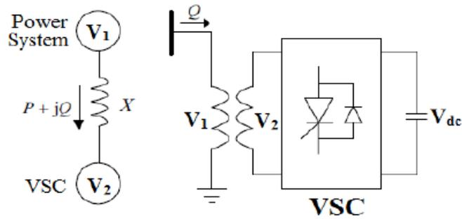
$V_1$  is the bus terminal voltage,  $V_2$  is the output voltage of STATCOM,  $V_{dc}$  is the DC capacitor side voltage,  $X_L$  is the inductive reactance, and  $\delta$  is the phase angle of  $V_1$  with respect to  $V_2$ .
