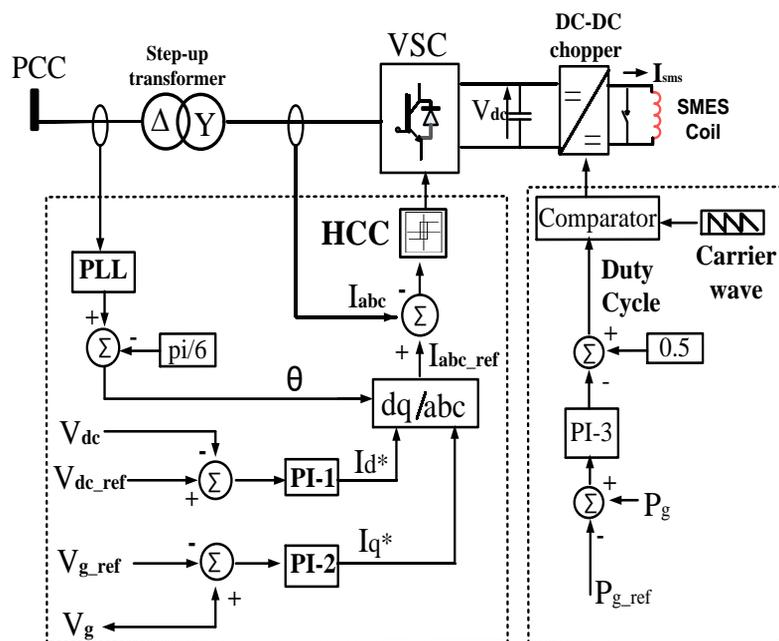
The superconducting coil is charged or discharged by adjusting the average voltage,  $V_{sms\_av}$ , across the coil which is determined by the duty cycle (D) of the two quadrant DC-DC chopper. To determine the value of the duty cycle of the DC-DC chopper, the power generation is used as input to a proportional integral (PI) controller. Based on this concept, the control system of a DC-DC chopper is
