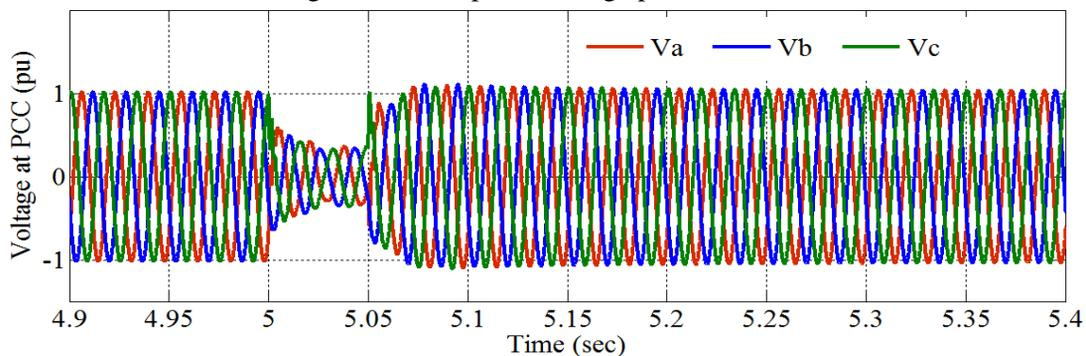
Figure 7: Voltage profile at PCC
